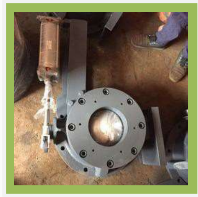
Water Cooled Dome Valves
